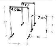
Obstacle 3 – The Floating Squares- made of 1/2" PVC Pipe and measurements are the opening size.
