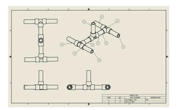
Obstacle 1 – The Shelf -made of ½" PVC Pipe and a piece of ½" plywood
