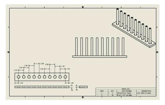
Obstacle 3 – Hills and Valleys- Made of wood mounted to a piece of  $\frac{1}{4}$ " plywood. Alternatively, the hills may be 3d printed and placed on  $\frac{1}{4}$ " plywood.
